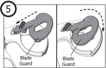
Flip over the handle. Insert the lever part of the **blade guard** into the handle. Lay it flat and extend the guard to lock it in place.
