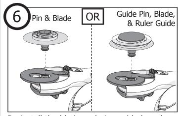
Re-install the blade and pin, or blade, ruler guide, and guide pin.
